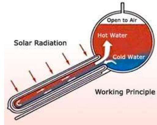
Especially in winter, vacuum collectors, due to their good insulation, obtain a significantly higher thermal performance than flat-plate solar collectors. Very low [temperature](#) resistance is given as an average of -30 degrees [Celsius](#).
