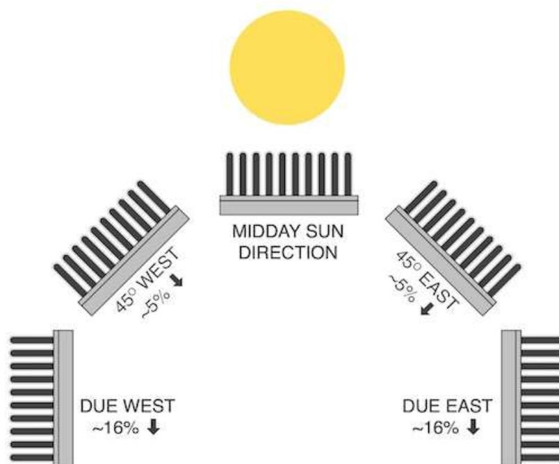
The Evacuate Tube collector has minimal power loss when the installation azimuth is out of optimal (out of south direction) – Flat Plate collector loses over half of its power and daily consumption.
